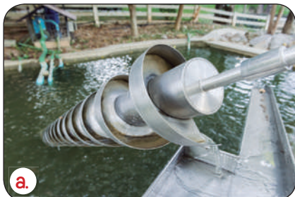
a. Archimedes’ screw. Archimedes. Greece, around 250 B.C.
